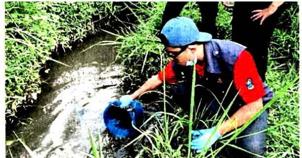
A Lembaga Urus Air Selangor worker collecting a water sample from a section of Sungai Gong close to an industrial area in Kuala Lumpur. PIC COURTESY OF LEMBAGA URUS AIR SELANGOR
